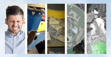
Deterioration can be accelerated by conditions that can occur during normal operations, such as debris on the impeller, blades, and/or housings. Other common factors include loose fasteners, improper maintenance, and deterioration due to normal outdoor climate conditions including rain, snow, sun, and salt.
